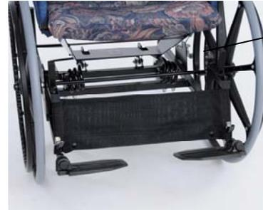
There are four inches of adjustment available with the footrest mounted in the lower mounting bracket on the base of the chair; more can be achieved by moving the footrest from the lower to the upper mounting bracket.
